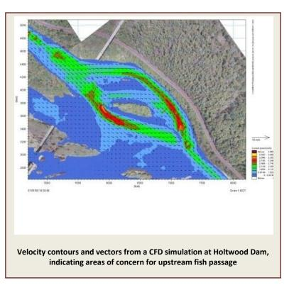
dam were modeled to evaluate the ability of deflector walls to minimize these problems. The end result of this modeling was that a design was developed that was suitable for approval by the regulatory agencies.
