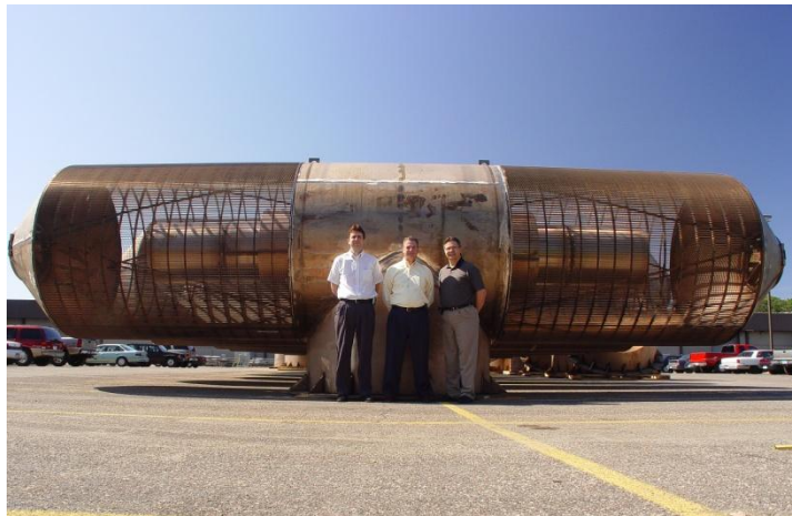
Figure 2 Cylindrical wedgewire screen used as an exclusion technology (courtesy We Energies)
