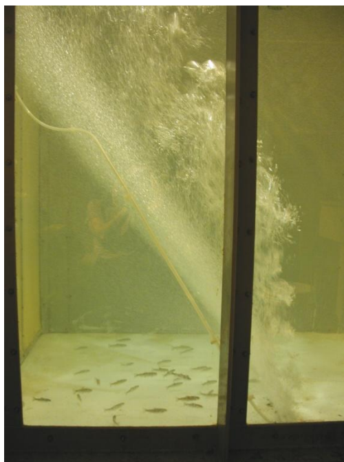
Figure 1 Laboratory evaluation of an air bubble curtain used as a behavioural technology for preventing entrainment of fish (courtesy Alden Research Laboratory)
