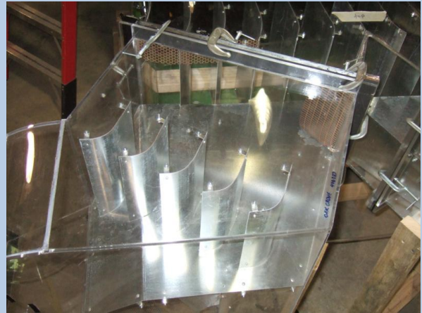
Figure 4: Flow controls in the absorber duct
