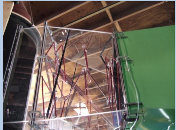
Figure 5: Modeled liquid collection system downstream of the absorber (right) and into the stack breach (left). The angle brackets can be seen in black, attached to the acrylic walls.
