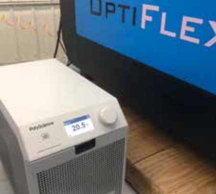
The PolyScience DuraChill connected to a Kern laser provides reliable temperature control.
