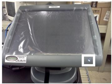
The power button is under the power light. Tilt workstation back:
