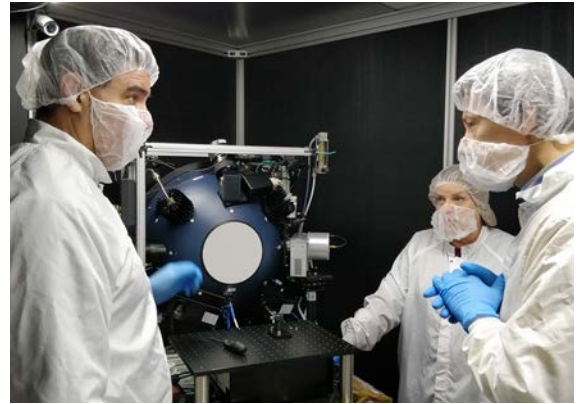
Right: Figure 2 NASA scientists paired the EQ-400 LDLS with an integrating sphere to ensure uniform output.
