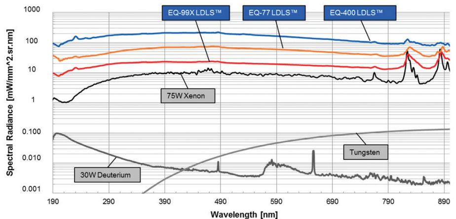
*The spectral radiance (brightness) of the LDLS exceeds that of traditional Tungsten sources across the UV-Vis-NIR spectral range as shown in Figure 2.*
