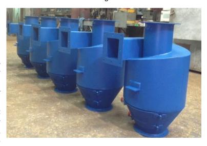
product, which is crucial in an application such as this where there are FDA regulations and all of the dust must be accounted for. Additionally, the GPC is more low maintenance than cartridge collectors. By sending the bulk of the application into the dust collector before the cartridge filter helps maintenance time and costs are drastically reduced.
