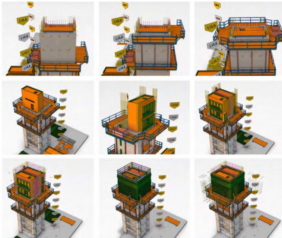
**Timber Tools** | Corrected sequence for formwork installation enabled through 3D simulation.
