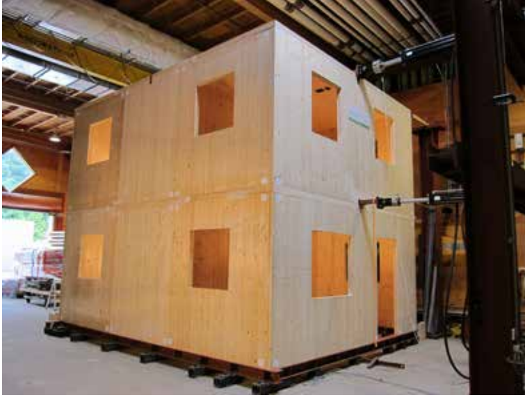
Figure 9 CLT test assembly at FPInnovations
