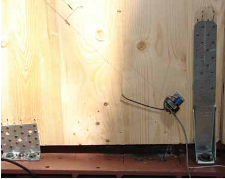
Figure 22 Behavior of one corner of Wall 08A during testing
