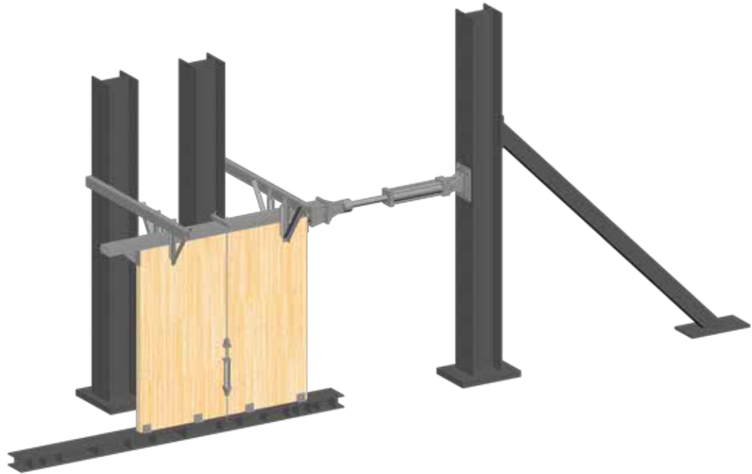
Figure 13 Test setup used for CLT walls
