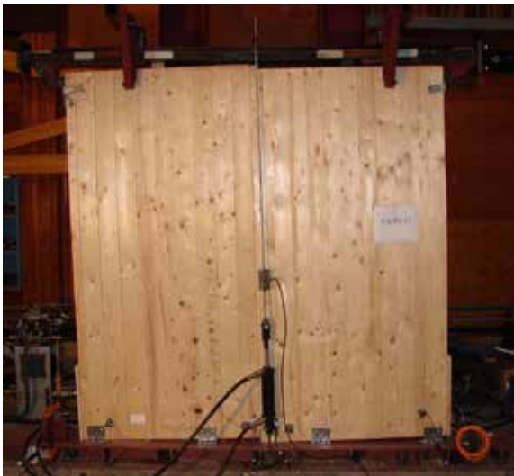
Figure 24 Behavior of Wall 12 using two panels during testing
