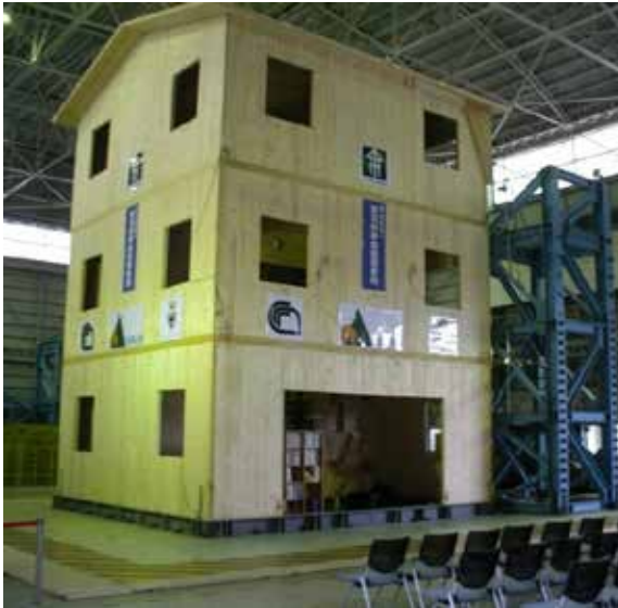
Figure 9 Three-story CLT house tested at NIED Laboratory in Tsukuba, Japan
