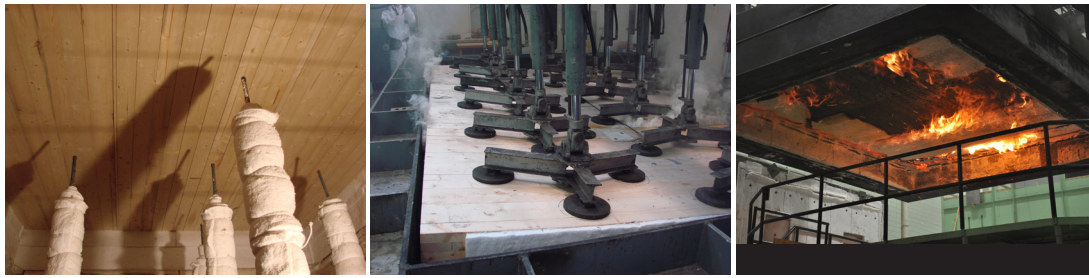
a) Unprotected CLT before test b) Unexposed surface during test c) Protected CLT after test
