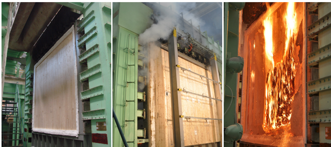
a) Unprotected CLT before test b) Unexposed surface during test c) Protected CLT after test
