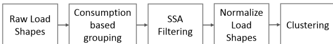
Fig. 1: The intermediate steps in the preprocessing procedure from the raw data load shapes to the clustering algorithm.
