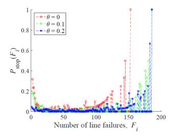
Fig. 2. The cascade-stop probability  $P_{\rm stop}(F_i)$  as estimated from simulation results. (Figure is adopted from [15].)
