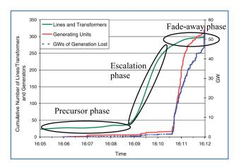
Fig. 1. Time evolution and the associated three phases of the cascading failure in 2003 Northeast US blackout. (Figure is adopted from [28].)
