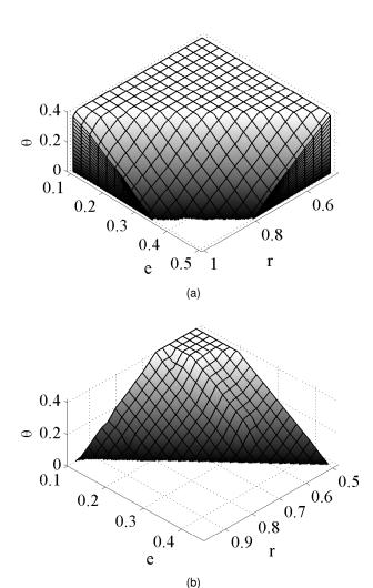
Fig. 6. Non-critical region for power-grid operating characteristics when (a) the impact of human behavior is not considered, and (b) the impact of human behavior is considered.
