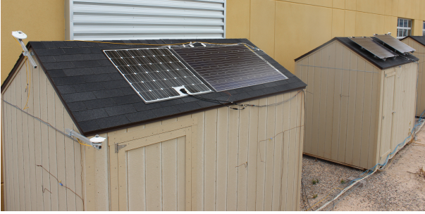
Fig. 1. The adhesively mounted glass-glass module is attached to the left test hut. The 4-inch and 7-inch mounted glass-glass modules are attached to the right test hut. The plane of array (POA) pyranometer is fixed on the left side of the left test hut.
