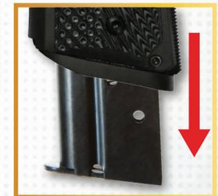
Place your free hand under the magazine to prevent it from falling and press the magazine catch to release and eject the magazine. Check the chamber for an un-extracted shell or unfired cartridge and remove such from the chamber. Press the slide stop down to allow the slide to move forward to its normal position. The pistol is now unloaded.
