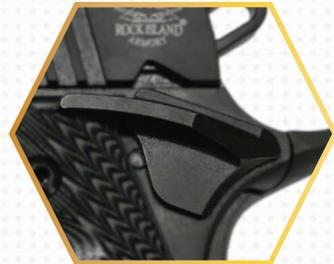
**THUMB SAFETY** - this is the manual safety located at the upper rear of the grip frame so the thumb of the shooting hand can be used to easily engage or disengage it, which can only happen when the hammer is fully cocked. When up and engaged, it blocks both the sear and hammer to prevent the gun firing. When engaged, this safety also blocks movement of the slide. The “cocked and locked” carry condition is achieved when the thumb safety is engaged.
