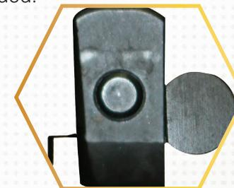
**INERTIA FIRING PIN** - the firing pin, designed to be shorter than its housing, is held to the rear by a spring and is intended to protrude to hit a cartridge primer only when a sufficient hammer blow overcomes the spring force and the inertia of the firing pin.
