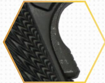
**GRIP SAFETY** - this safety blocks rearward movement of the trigger in order to prevent the gun firing unless the grip safety is first disengaged by the firm grasp of the shooting hand in normal shooting position, thereby allowing complete rearward trigger movement.
