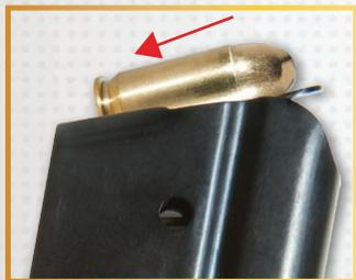
Grasp magazine in one hand and place a round on the magazine follower with the base of shell first and push down. Let the cartridge slide under the feed lips until base of cartridge touches the flat edge of the magazine. Place next round on top of previous round, press down again and into back. Repeat until the magazine is loaded to its rated capacity. Do not exceed capacity.
