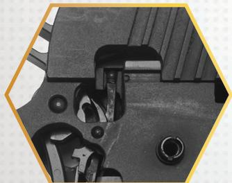
**DISCONNECTOR** - this device interrupts the activation of the sear by the trigger in order to prevent the sear from releasing the hammer to fire a chambered cartridge until the slide and barrel are locked together and the trigger is released and pulled again.
