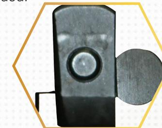
**INERTIA FIRING PIN** - the firing pin, designed to be shorter than its housing, is held to the rear by a spring and is intended to protrude to hit a cartridge primer only when a sufficient hammer blow overcomes the spring force and the inertia of the firing pin.
