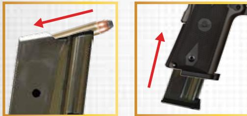
To load the magazine, place the first cartridge in the front end of the magazine follower and push it down until it can be slid in under the feed lips of the magazine. Place the second cartridge on top of the first and force it down in the same way as the first one. Repeat this procedure until the magazine contains the number of cartridges you intend to load. (Note: Refer to the specification for the magazine capacity).
