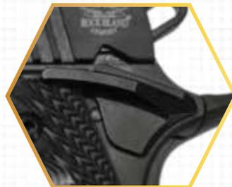
**THUMB SAFETY** - this is the manual safety located at the upper rear of the grip frame so the thumb of the shooting hand can be used to easily engage or disengage it, which can only happen when the hammer is fully cocked. When up and engaged, it blocks both the sear and hammer to prevent the gun firing. When engaged, this safety also blocks movement of the slide. The "cocked and locked" carry condition is achieved when the thumb safety is engaged.
