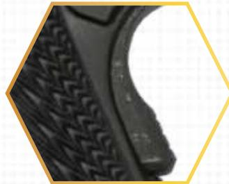
**GRIP SAFETY** - this safety blocks rearward movement of the trigger in order to prevent the gun firing unless the grip safety is first disengaged by the firm grasp of the shooting hand in normal shooting position, thereby allowing complete rearward trigger movement.
