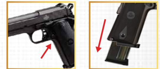
To unload, press the magazine release and remove the magazine. If the slide is in the forward position, pull it to the rear and retain by pushing the slide stop up. Inspect the chamber to make sure that the pistol is clear and unloaded. If there is a shell or unfired cartridge in the chamber, manually remove it before pressing the slide stop down. Your gun is now unloaded.
