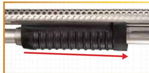
When gun is fired, action automatically unlocks. Forearm can be fully drawn back and pushed forward. This extracts and ejects fired shell through ejection port opening facing downward.
