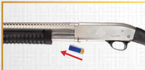
With trigger locked, insert shell upward into bottom of receiver and push forward into magazine tube past cartridge stops. Repeat until magazine tube is full.
