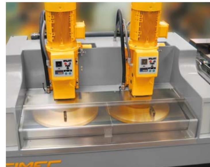
In order to satisfy the needs of customers who carry out versatile productions, SIMEC also makes the LM 2100 RX in a combined version for the calibrating, dressing and polishing of small slabs or strips. An effective, compact solution for obtaining perfectly calibrated and polished material with just one machine. This operation is performed by means of rotating plates fitted with diamond tools, installed in a fixed position.
