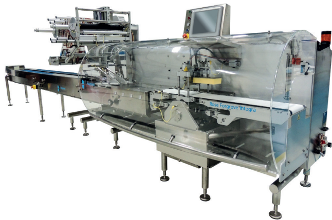
This horizontal packaging unit is used for products that need a long shelf life
