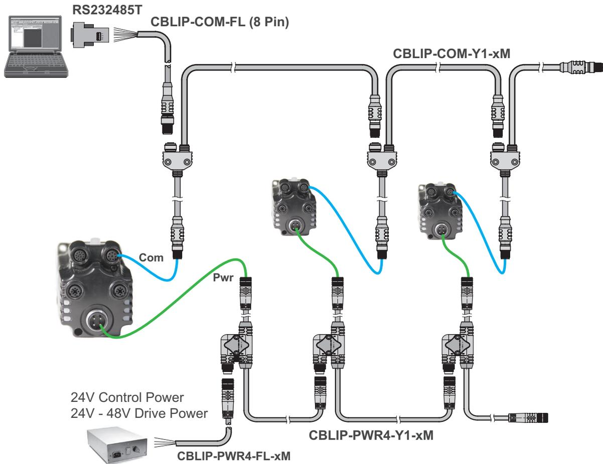
**NOTE:** RS-485 serial communications uses a voltage differential signal that requires proper termination with a 120 ohm resistor across pins 2 and 3 at both ends of the network cable. This follows RS-485 standards for biasing to ensure reliable performance. The termination can be created by adding the resistor to CBLIP-COM-FL Flying Lead cables or to off-the-shelf connectors.
