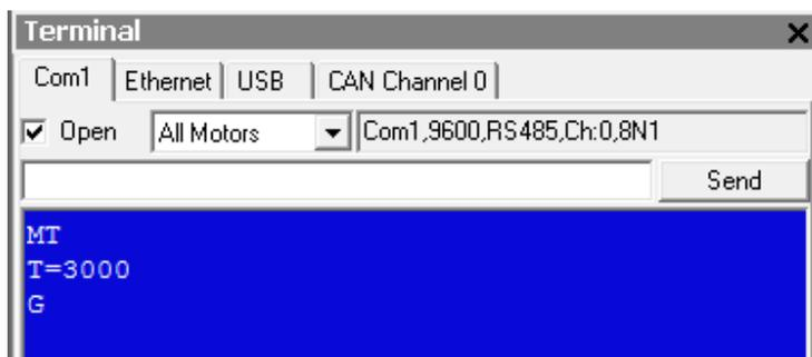
You should immediately see the motor shaft moving in the positive direction (clockwise, when looking at the end of the motor shaft). If the motor does not respond to the commands, see Troubleshooting on page 54 for troubleshooting tips.
