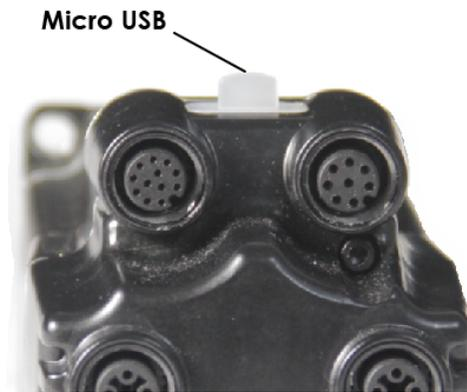
*Micro USB Connector (Located Under Protective Cover)*
