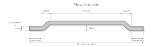
A typical rod anchor has a 1/4" diameter, and a total rise of 5/8" (1/4" diameter plus the rise of 3/8") off of the steel member it is welded to. The purpose of the rise is to provide a mason with room to install an insert that will join with a concrete or brick wall.
