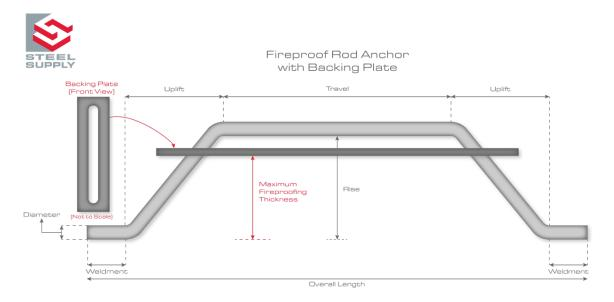
The only drawback of the backing plate is that simply rest on fireproof anchor rods that have 90 degree. If a backing plate is used in this case, it will require a tack weld.
