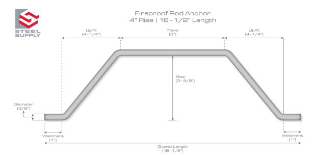
If a specific **travel** length is required in a limited space, the **uplift** of the **fireproof rod anchor** can be adjusted to a 90 degree angle, which decreases the **overall length**. Additionally, the following two diagrams show that the **weldments** can be pointed to the outside of the rod anchor, or to the inside. This is another option that accommodates tighter spaces.
