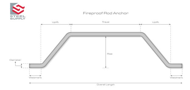
While a normal rod anchor is made with 1/4" diameter steel, a fireproof rod anchor is generally made with a 3/8" diameter. This is done to mitigate the deflection that would be caused in the steel as a result of the increased length in the uplift and travel of the rod anchor. With a 3/8" diameter, the yield strength of the steel increases by 2.24 times when compared with the same rod of a 1/4" diameter.
