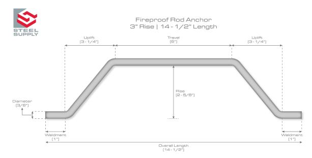
In many cases, a rod anchor will need to be welded specifically to a column, and this is also the case for fireproof rod anchors. If the fireproof rod anchor is to be mounted to a column, the dimensions are practically inconsequential. A fireproof rod anchor of any dimensions will work. However in the case of a horizontal beam, it is not uncommon for the rod anchor to be mounted inside of its web. In these cases, overall length is a substantial factor.
