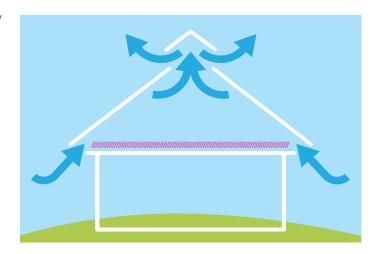
Soffit vents should be located as far to the outside edge of the soffit as possible. Otherwise, warm air next to the heated siding can rise, enter the vent, melt snow, and contribute to ice dams forming.
