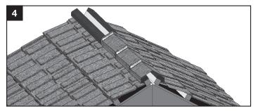
Install the appropriate Hip and Ridge pieces over the vent material. Fasten the screws through the vent material into the battens.
