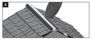
Remove the 1x4 spacer and roll out the vent material along the tops of the battens. Remove the white paper while unrolling to expose the adhesive dots. Apply pressure over the adhesive dots to hold the material in place during installation.
