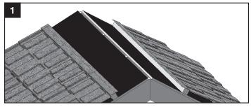
Install panels up to last full course before ridge according to installation instructions. Cut both sides of the plywood 3/4 inch from the center of the ridge to expose attic space.
