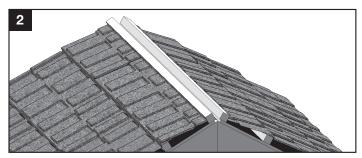
Install wood battens along the ridge. Align the top edge of the 2x2 along the edge of the plywood on both sides of the ridge to expose the attic opening. Measure, cut, bend, and install the final course of panels.
