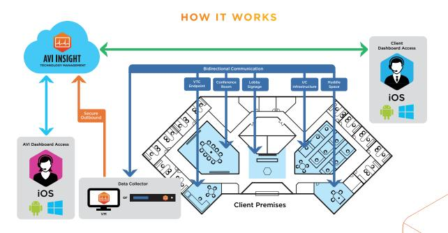
AVI Insight relies on a server, or "data collector," that resides on the client's network. The data collector monitors all networked devices and communicates essential data to AVI Insight via a secure outbound socket. The data collector is the ONLY device that communicates outside the client network.
