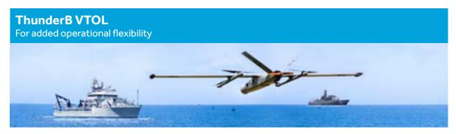
A dual-hybrid version, the ThunderB Vertical Takeoff and Landing (VTOL) can take off vertically from a very small patch of ground or marine vessel using its quad vertical electrical motors. Its transition to a level flight is powered by a high endurance horizontal fuel-injection engine, and after fulfilling its operational mission, it transitions back to a precise, vertical landing that requires a much smaller logistical footprint as compared to a standard launch and recovery system.
