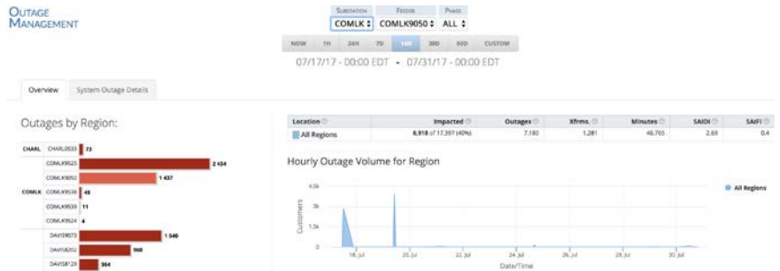
The above illustration shows outage duration, in minutes, by feeder and region
