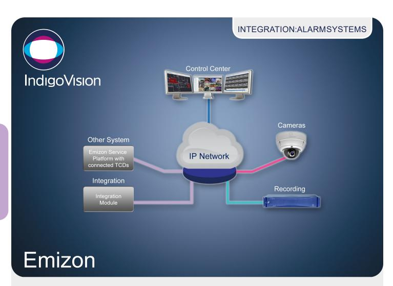
The IndigoVision Emizon Integration Module allows alarms and events from the Emizon Service Platform to be seamlessly combined with IndigoVision's video security solution, giving complete video and alarm management in a single user interface – Control Center.
