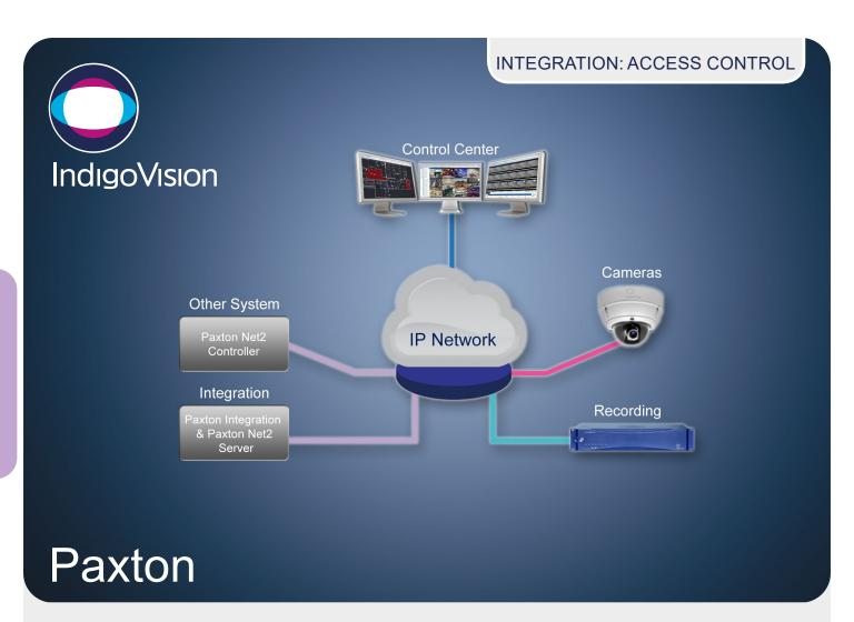
The IndigoVision Paxton Integration allows alarms and events from Paxton Net2 systems to be seamlessly combined with IndigoVision's video security solution, giving complete video and alarm management in a single user interface – Control Center.
