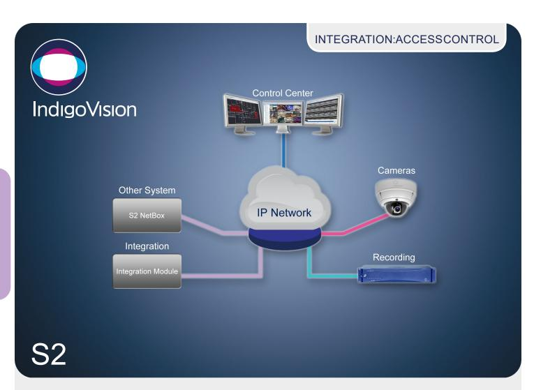
The IndigoVision S2 Integration Module allows alarms and events from the S2 Netbox system to be seamlessly combined with IndigoVision's video security solution, giving complete video and alarm management in a single user interface – Control Center.
