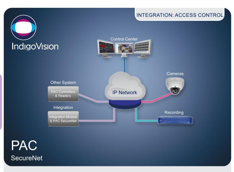
The IndigoVision PAC SecureNet Integration Module allows alarms and events from PAC systems to be seamlessly combined with IndigoVision's video security solution, giving complete video and alarm management in a single user interface – Control Center.
