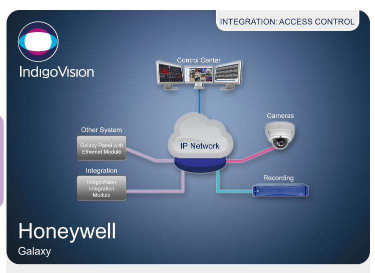
The IndigoVision Honeywell Galaxy Integration Module allows alarms and events from the Honeywell Galaxy system to be seamlessly combined with IndigoVision's video security solution, giving complete video and alarm management in a single user interface - Control Center.
