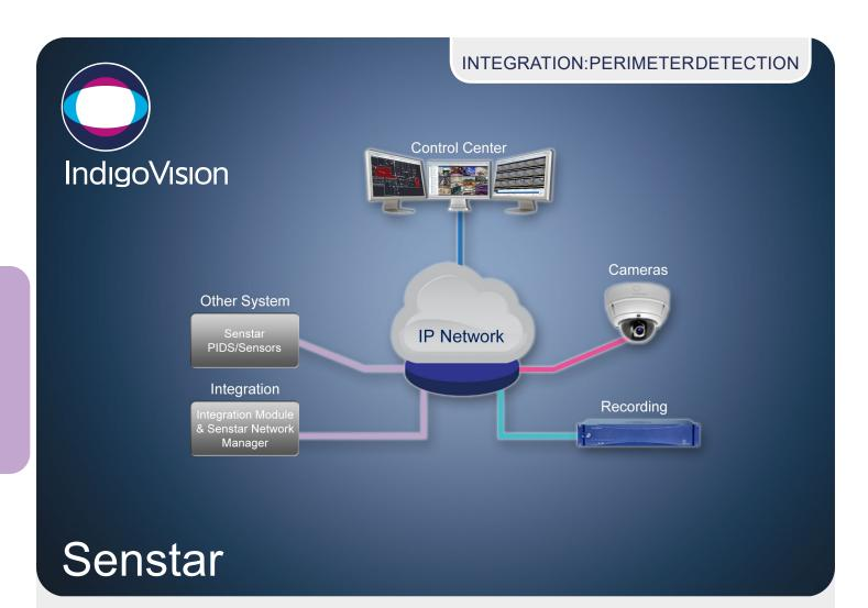
The IndigoVision Senstar Integration Module allows alarms and events from Senstar systems to be seamlessly combined with IndigoVision's video security solution, giving complete video and alarm management in a single user interface – Control Center.
