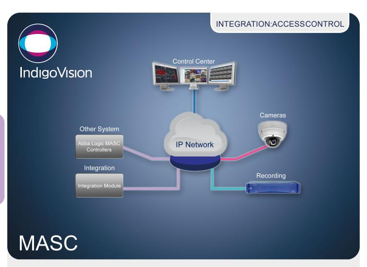
The IndigoVision MASC Integration Module allows a bi-directional flow of events and alarms between the Abba Logic MASC system and IndigoVision's video security solution.
