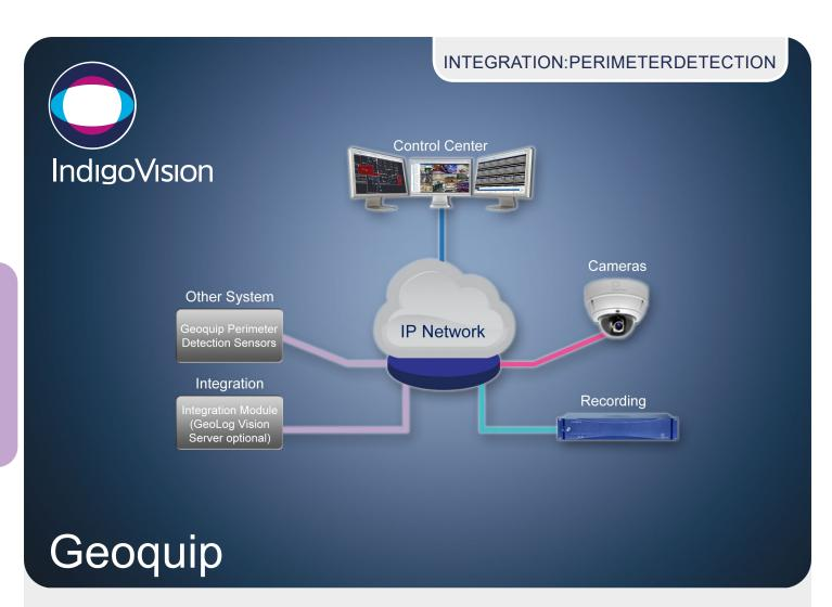
The IndigoVision Geoquip Integration Module allows alarms and events from the Geoquip system to be seamlessly combined with IndigoVision's video security solution, giving complete video and alarm management in a single user interface – Control Center.
