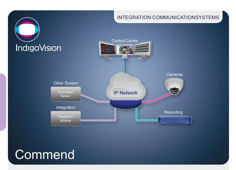
The IndigoVision Commend Integration Module allows events from the Commend intercom system to be seamlessly combined with IndigoVision's video security solution, giving complete video and alarm management in a single user interface – Control Center
