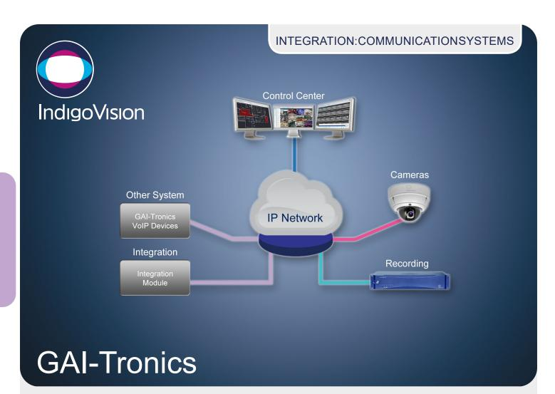
The IndigoVision GAI-Tronics Integration Module allows alarms and events from GAI-Tronics VoIP devices to be seamlessly combined with IndigoVision's video security solution, giving complete video and alarm management in a single user interface – Control Center.
