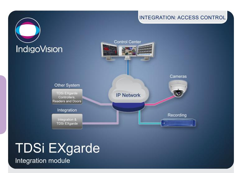
The IndigoVision TDSi EXgarde Integration allows alarms from TDSi systems to be seamlessly combined with IndigoVision's security management solution, giving complete video and alarm management in a single user interface – Control Center.
