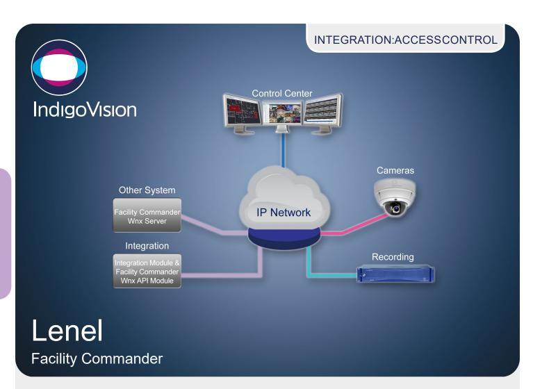
The IndigoVision Facility Commander Integration Module allows a bi-directional flow of events and alarms between Facility Commander Wnx and IndigoVision's video security solution, giving complete video and alarm management in a single user interface – Control Center.
