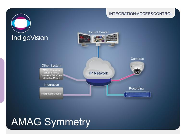
The IndigoVision AMAG Symmetry Integration Module allows a bi-directional flow of events and alarms between AMAG Symmetry and IndigoVision's video security solution, giving complete video and alarm management in a single user interface – Control Center.
