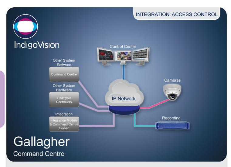
The IndigoVision Gallagher Integration Module allows seamless two-way communication of alarms and events between the Gallagher Command Centre System (formerly Cardax) and IndigoVision's Control Center suite.
