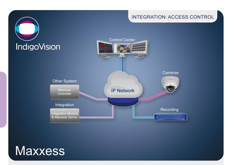
The IndigoVision Maxxess Integration allows alarms and events from Maxxess systems to be seamlessly combined with IndigoVision's security management solution, giving complete video and alarm management in a single user interface – Control Center.
