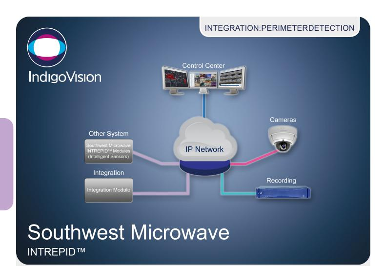
The IndigoVision Southwest Microwave Integration Module allows alarms and events from the Southwest Microwave INTREPID™ system to be seamlessly combined with IndigoVision's video security solution, giving complete video and alarm management in a single user interface – Control Center.
