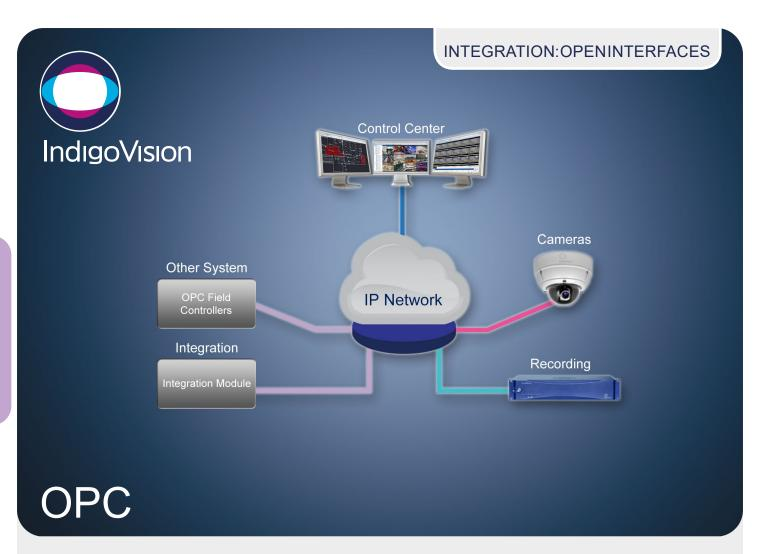
The IndigoVision OPC Integration Module allows a bi-directional flow of events and alarms between any other system providing an OPC interface and IndigoVision's video security solution. Events and alarms can also be managed with one-click acknowledgements from within the third party software.
