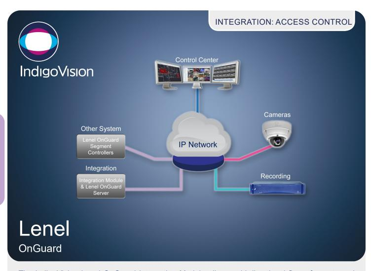
The IndigoVision Lenel OnGuard Integration Module allows a bi-directional flow of events and alarms between Lenel's OnGuard system and IndigoVision's video security solution.
