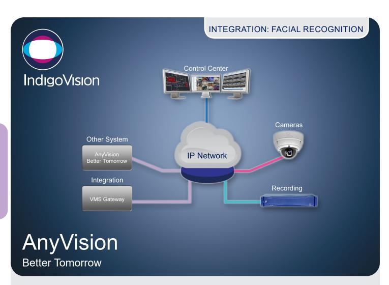
The AnyVision Integration Module allows face recognition events from AnyVision's Better Tomorrow system to automatically trigger real-time events in IndigoVision Control Center, as well as generating data records which index recorded video with time-stamped information.
