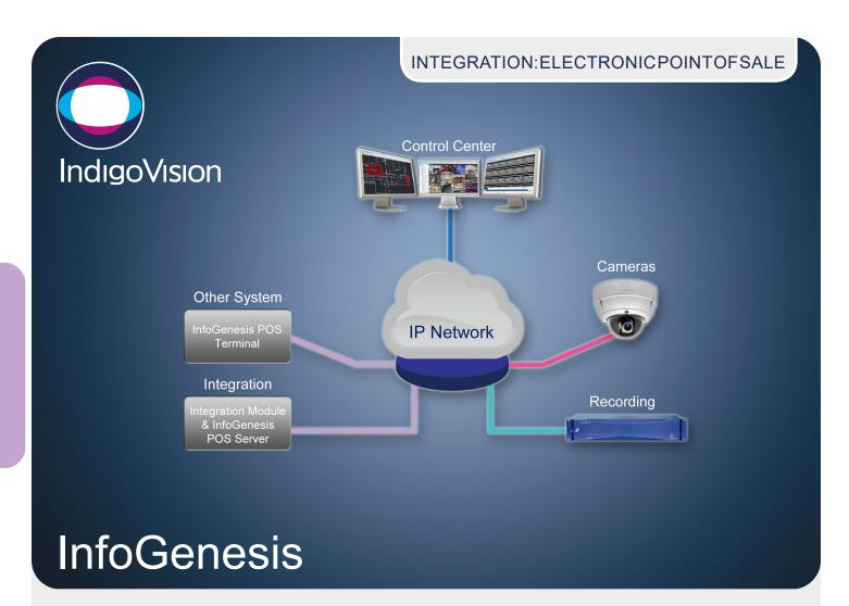
The IndigoVision InfoGenesis Integration Module allows a flow of events and alarms from the InfoGenesis Point of Sale (PoS) system into IndigoVision's video security solution.
