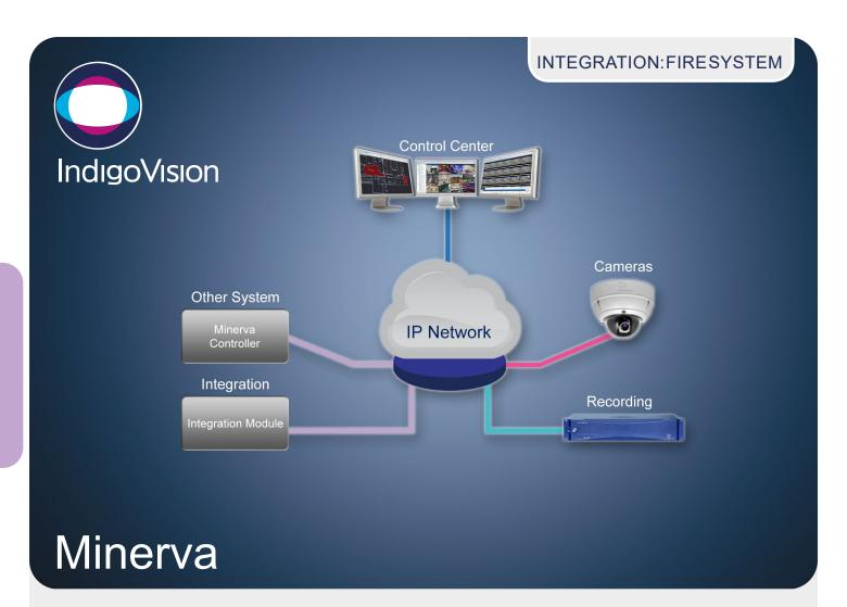
The IndigoVision Minerva Integration Module allows alarms and events from Minerva controllers to be seamlessly combined with IndigoVision's video security solution, giving complete video and alarm management in a single user interface – Control Center.
