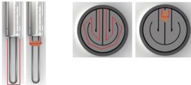
Figure 6 Bridging may shorten electrical paths, and affect accuracy of ER corrosion probes measurements. 7
