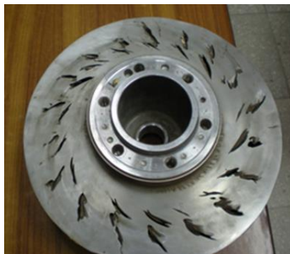
Figure 4 A damaged impeller.
