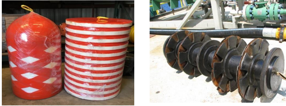
Figure 10 Maintenance pigs used to displace liquids (left) or scrape/clean multi-diameter pipelines (right).
