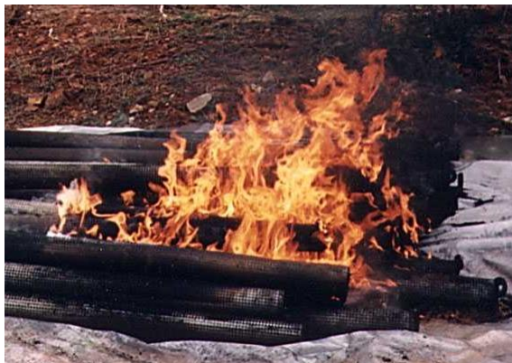
Figure 1 Cartridges, which collected pyrophoric iron sulfide, were allowed to dry – spontaneous combustion! 5
