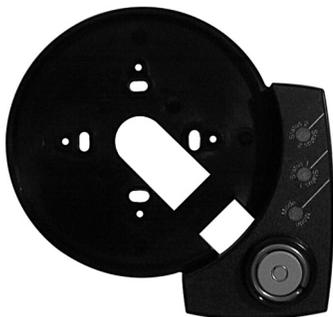
**Keypad Extension Base** — Installed under the keypad. This is required when using the lock’s Service Mode operation or audit trail function. The extension base provides a green LED to indicate “Status 1”, and a red LED to indicate “Status 2” and a yellow LED to indicate “Mode” of lock operation. The extension base also provides a port for communication with Touch Keys.
