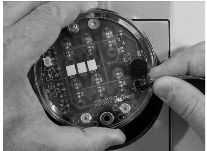
Line the two raised ribs on the connector with the matching slots in the receptacle, as shown.
