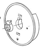
NOTE: If the lock is equipped with a tube, the dial ring bushing will seat over the end of the tube.
