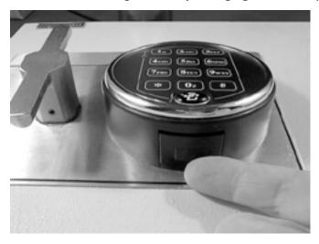
1. Keypad disassembly is neither required nor advised. The removable battery holder is accessed from the bottom of the keypad base. Pull it slightly toward the front of the keypad, then downward to remove it.
