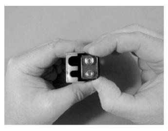
3. Note that the battery is oriented so that the larger contact is in line with the larger opening in the top of the battery holder. It's important to orient the new battery this way.
