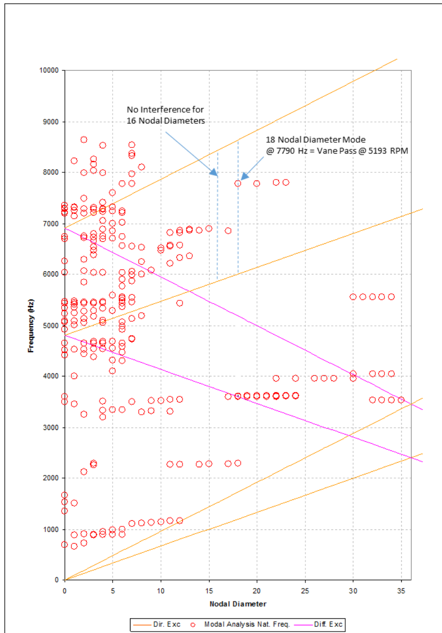
Figure 4. Potential problem mode was identified by using an Interference Diagram. As a result, the number of nozzle of the turbine was recommended to be reduced from 90 to 88 or less to avoid resonances. The pairs of diagonal lines represent the lower and upper speed ranges, respectively.
