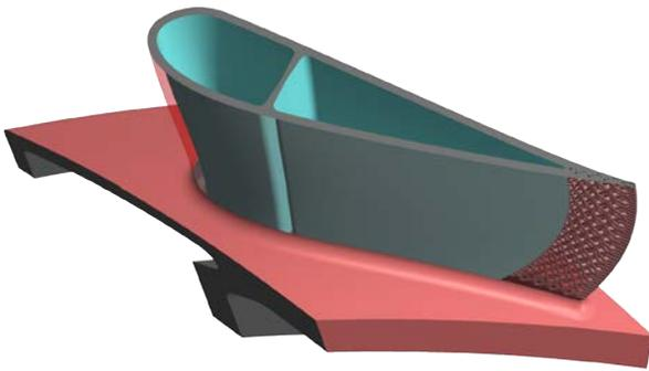
▲ Position of new channels within the blade
