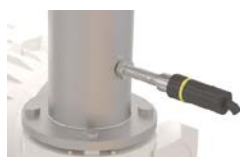
Option 2: RPM Sensor, Shaft reading
