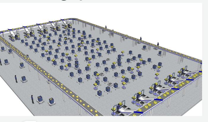
**Geek+ Sorting Robot** uses a strong AI algorithm and flexible system scheduling to figure out the most effective path and reduce convergence. The robot could do fast sorting automatically and send parcels to the corresponding shipment port.
