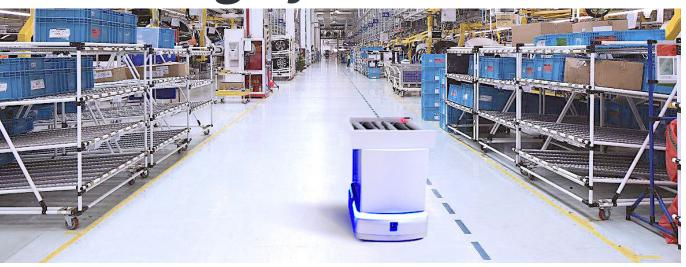
**Moving Robot** leverages advanced SLAM laser navigation method to identify factory's environment and schedule the route independently. The robots are able to avoid the obstacle to deliver pallet / rack to the destination in a flexible and smooth way.
