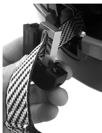
Ensure webbing is free of twists when aligning nozzle insert
