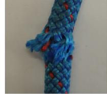
*Nicked or cut rope must be retired*
