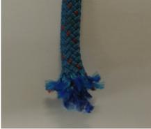
*Frayed ends must be properly terminated*
