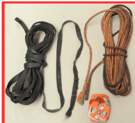
Routinely inspect lines, equipment, and hardware. The equipment pictured above would need to be removed from operation immediately and replaced.
