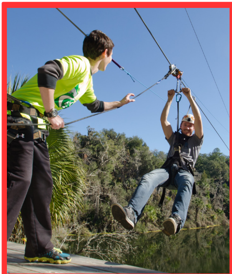
The Impact Trolley with pivoting handlebar is specially engineered to keep riders facing forward and out of reach of the zip line cable and impact areas.
