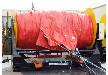
The Lamor Hydraulic operated Unireel 16 is designed to store up to 300 m length of up to max. 2200 mm oil booms like Lamor Uniboom X offshore booms. The maximum storage capacity for each size and type of boom must be confirmed with Lamor representative.
