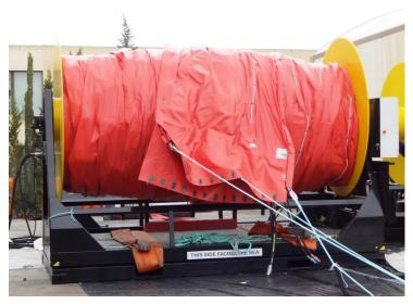
The Lamor Hydraulic operated Unireel 12 is designed to store up to 300 m length of max 1500 mm oil booms like Lamor Uniboom X offshore booms. The maximum storage capacity for each size and type of boom must be confirmed with Lamor representative.
