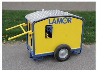
The Hydraulic Power Pack LPP 19 L/22cc is used as a power source for skimmers and other smaller hydraulically operated equipment such as boom reels, air blowers etc. The power pack is a light-weight, easily portable power solution for hydraulic equipment that can be operated in remote locations.
