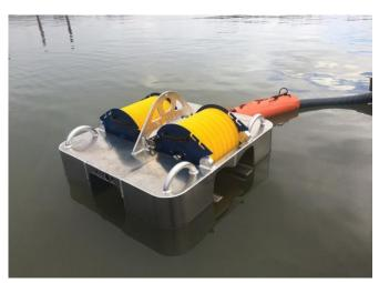
The compact Minimax 50 skimmer is a modular, robust oil skimming unit that is easily transported, assembled and cleaned.
