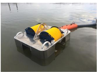
The compact Minimax 50 skimmer is a modular, robust oil skimming unit that is easily transported, assembled and cleaned. The skimmer frame is manufactured in marine grade aluminum.
