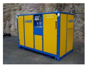
The Lamor Power Pack LPP 119 Cu/135cc is powered by a water cooled 119 kW Cummins 4.5 I turbocharged/intercooled diesel engine and serves as a high capacity multipurpose power pack designed for the flexible operation of many types of hydraulically operated oil spill clean-up equipment.
