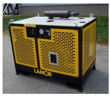
The Hydraulic Power Pack LPP 35 is used as a power source for skimmers and other hydraulically operated equipment such as boom reels, pumps etc. Equipped with 2 hydraulic circuits, the LPP 35 can power multiple pieces of equipment simultaneously (for example a skimmer and an oil transfer pump).
