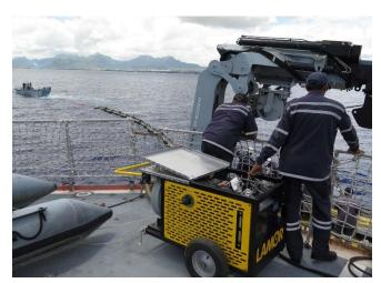
The Lamor Power Pack LPP 14 L with integrated air blower HAB 200 is a multipurpose power source that is ideal for deploying heavy duty and light inflatable oil booms from reels.
