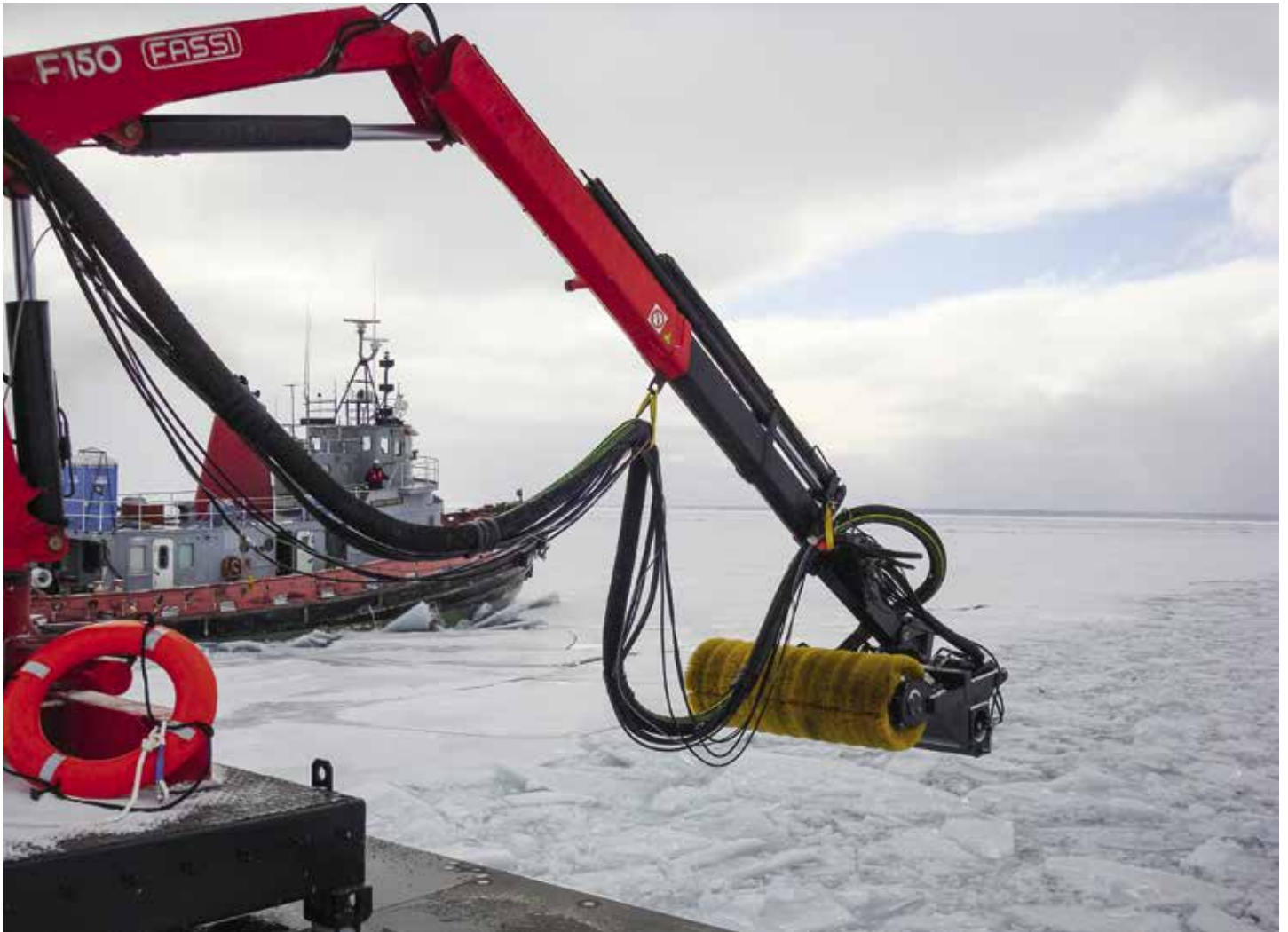
The Lamor Oil Recovery Bucket (LRB) can be effectively operated by a crane onboard a vessel or excavator.
