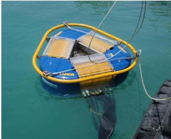
The Lamor Multi Skimmer LMS 115/140 is a flexible high capacity free-floating skimmer, which is designed with interchangeable brush, disc, and drum modules in a triangular configuration, suitable for a variety of different oil spill recovery scenarios. The LMS 115/140 is designed to recover oil from harbours and nearshore but also offshore. With all its options, the LMS 115/140 provides the user with several skimming options ranging from brush, disc and drum.
